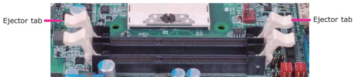
5. Note how the module is keyed to the socket.
